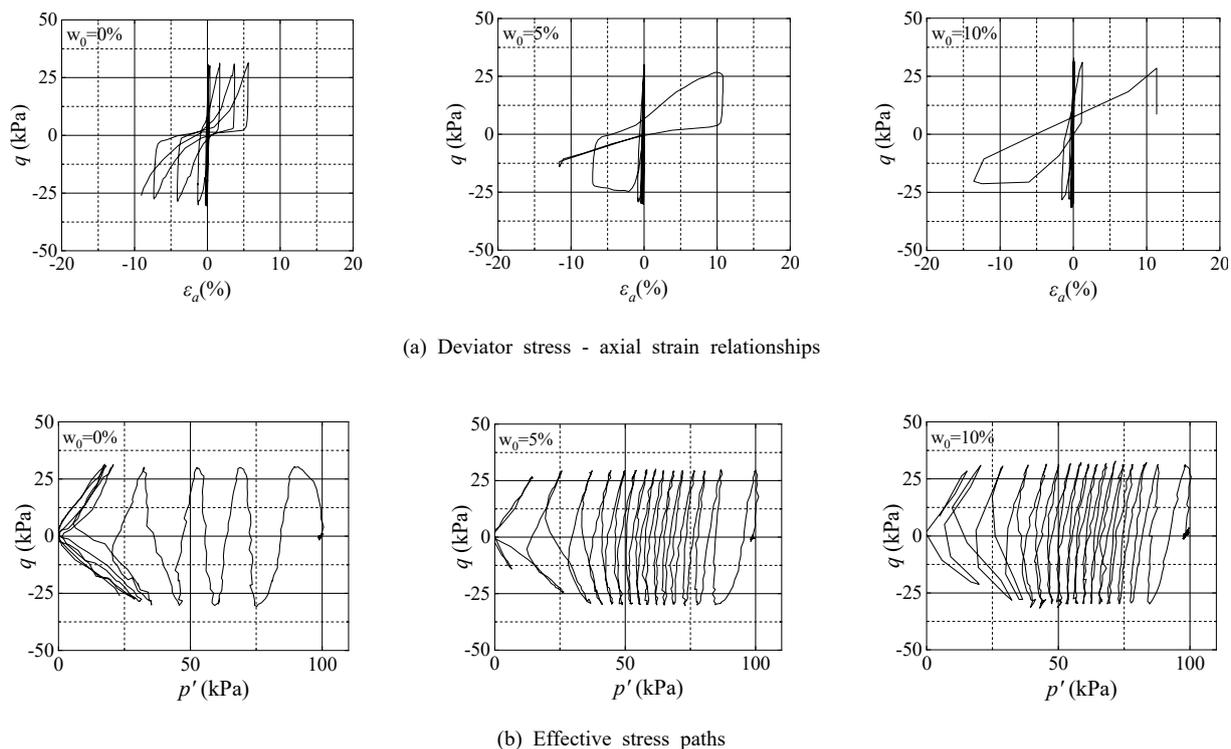
Figure 4. Test results of triaxial test under cyclic loading condition.
