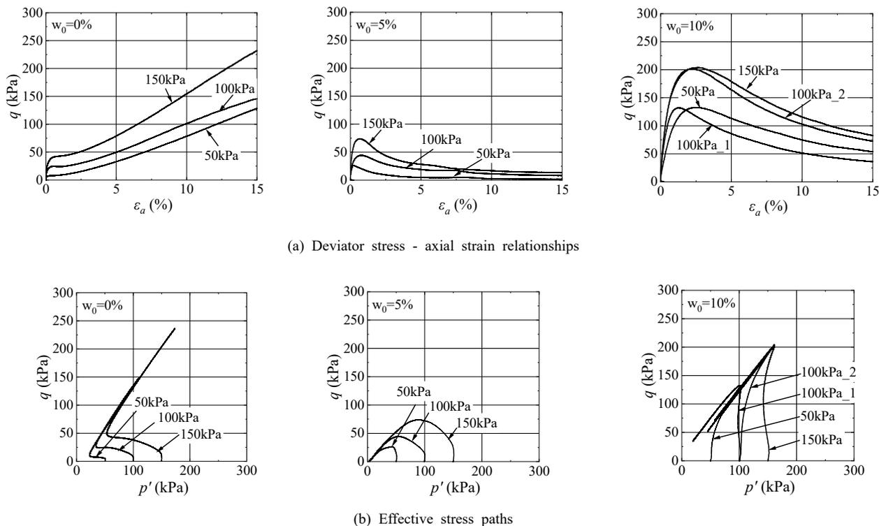
Figure 3. Test results of triaxial test under monotonic loading condition.
