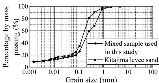
Figure 1. Grain size distribution of the test sample.
