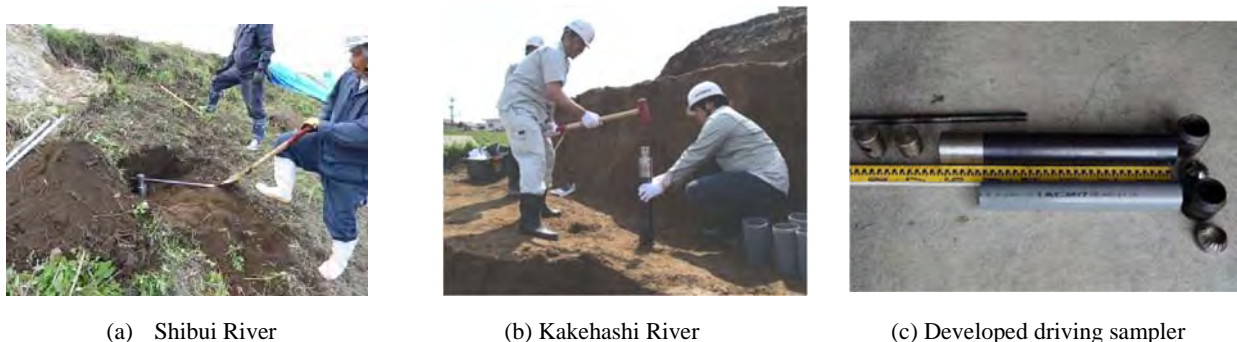
Photo 1. Situations of field sampling of embankment soils at actual levees by the simple sampling method.
